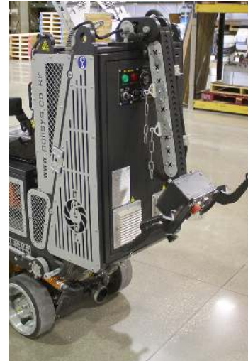
Lower Position: for remote operation and transportation
