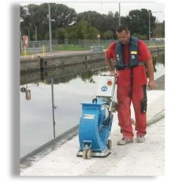
IMPACTS Americas, Inc. +1.815.941.4800 www.IMPACTSAmericas.com The IMPACTS S210E-40R is a very powerful, but compact and light weight mobile blast machine. The combination of the powerful wheel motor with an optimized separation system and the variable speed drive motor makes the machine very efficient.
