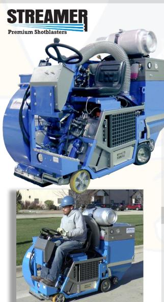
IMPACTS Americas, Inc. +1.815.941.4800 www.IMPACTSAmericas.com The S320RD Ride-on propane model is perfect for powerful shot blasting with the added convenience of a seat & steering wheel! At 12.6 inches and 24HP, the S320RD Streamer will out blast comparably-sized and priced blasting machines.
