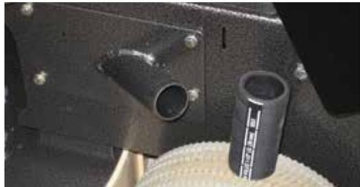
3. Use the strap and footman loop located on the side of the control panel to retain a vacuum hose against the machine during operation.
