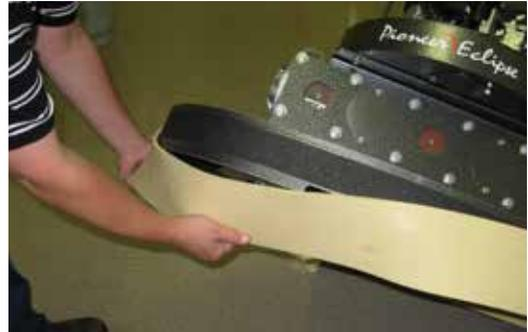
4. To re-install the skirt, start in the back and stretch the skirt over the perimeter of the deck.
