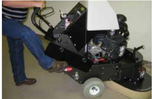
5. Rock the machine back by pushing down on one of the foot pegs while pulling back on the handle.
