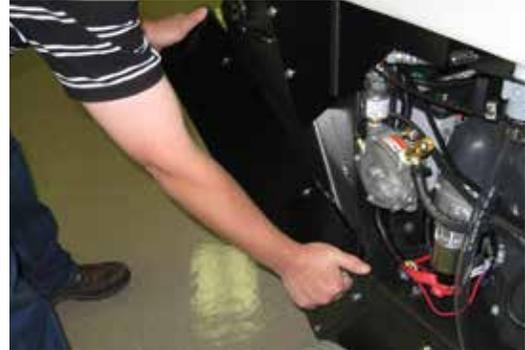
3. Place the handle in the head change position (see Handle Adjustment / Position section).
