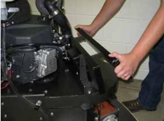
4. Hook the Transport handle to the bracket under the deck.
