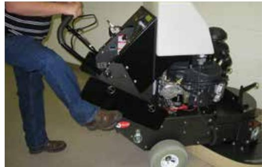
5. Push the machine around on the two rear wheels.
