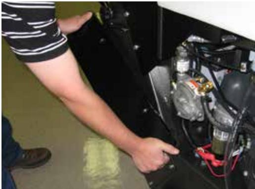
3. Remove any of the remaining weight plates from the front of the machine.
