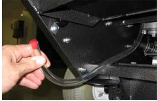
5. Place a suitable container under the end of the oil drain hose.
