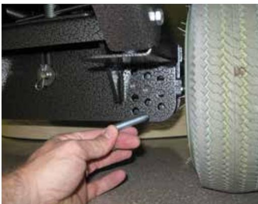
7. Using the axle height adjustment "T" handle, adjust the height of the axle to the desired position.
