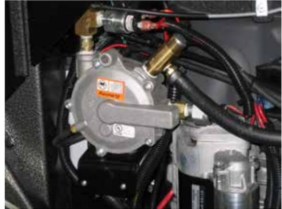
5. If a leak is detected, turn off the LP cylinder. If the leak is in a hose, replace it. If the leak is at a fitting, loosen and clean it. Apply pipe-sealing compound and re-tighten it.
