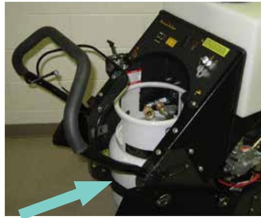
**CAUTION!** Always open service valve slowly to allow pressure to equalize in hoses. Opening quickly may cause the flow check valve to engage, limiting fuel flow.
