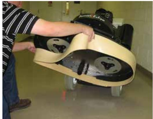
5. When the bottom edge of the skirt is worn, the skirt can be removed and flipped over to provide a new wear edge.
