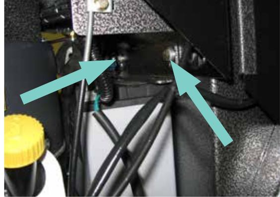
3. Disconnect the BLACK negative battery cable first. Disconnect the RED positive battery cable last.
