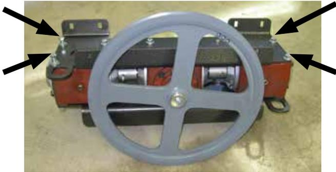
2. Remove the shear pin from the coupling of the gearbox being replaced.
