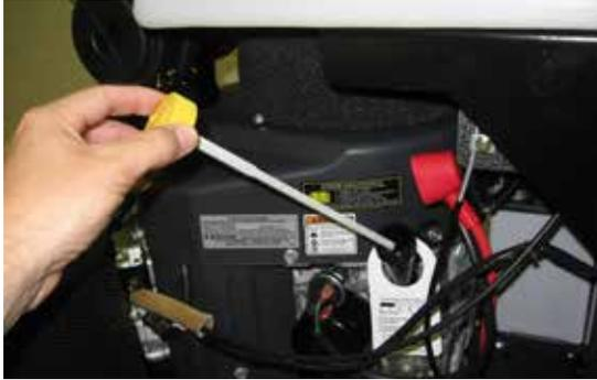
5. The machine should be in an upright level position.
