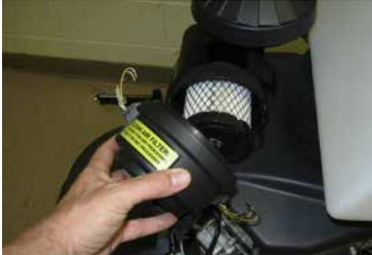
6. Inspect the air cleaner. If necessary, clean the filter by lightly tapping and wipe seal ends with a clean cloth. If the filter cannot be cleaned, bent, or damaged, it must be replaced. (**Part #: KA110137048**)
