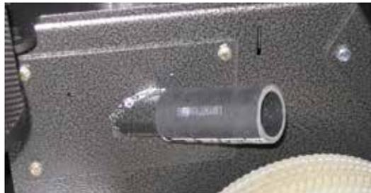
2. To connect a 1-1/2" diameter hose to the port, the adapter must be removed. Leave the adapter for a 2" diameter hose.
