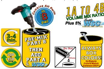
Mix combined components of Smith's Epoxy VCB38 for 3 to 4 minutes using a low speed (≤450 RPM) 1/2" drill using a paint mixing paddle in a plastic 5 gallon pail. DO NOT MIX MORE MATERIAL THAN CAN BE USED WITHIN 25 MINUTES AT 72°F. Once Part B is pigmented with Smith's WSC Color Packs, it must be used within the same day.
